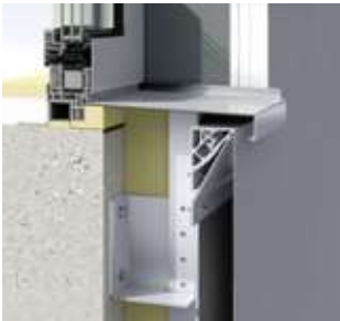
Fassadendetail Fensteranschluss Façade section detail, window attachment
